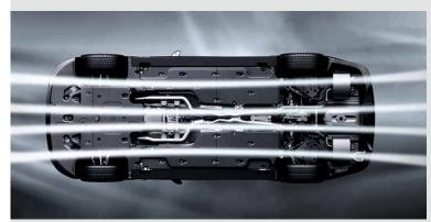
**Multiple undercovers and aerodynamic effects** While the aerodynamic aspects of the silhouette are plain to see, the All-New Stinger also boasts vital drag reduction features that improve airflow underneath the car. It uses a system of sturdy undercovers, below the engine and transmission, each side of the cabin and each side of the rear suspension. These covers reduce the flow resistance on the underside of the body when travelling at higher speeds.
