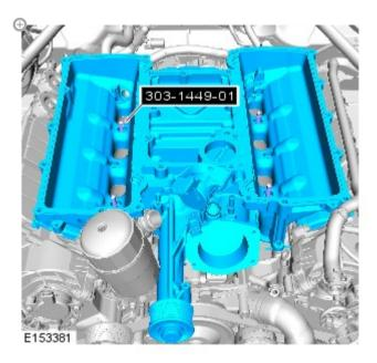
Install the supercharger assembly.
